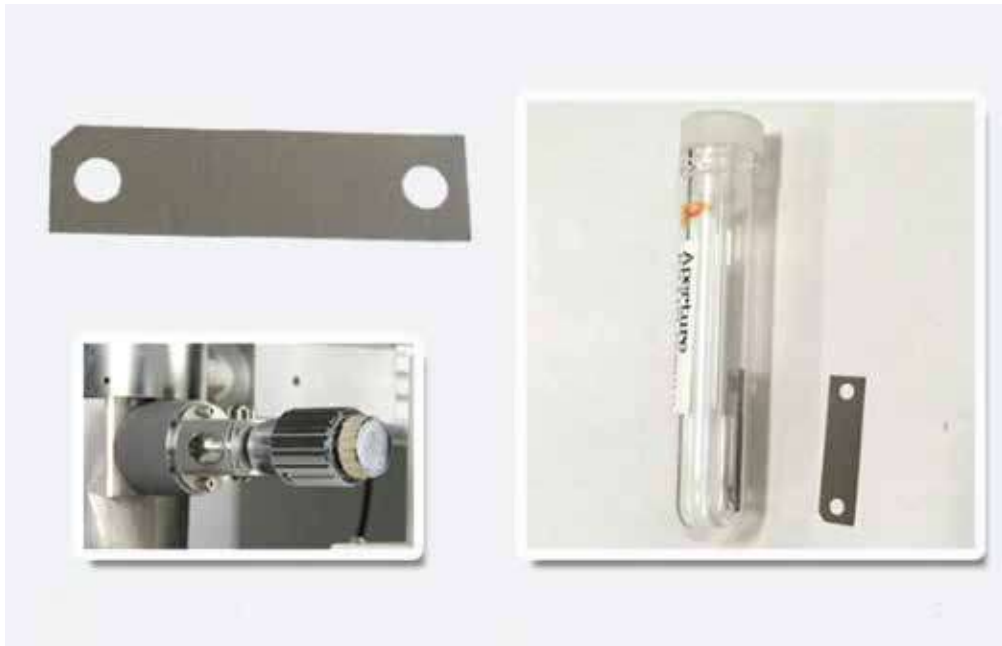
The Aperture Plate Has Three Nano-sized Holes Through Which Light Passes
